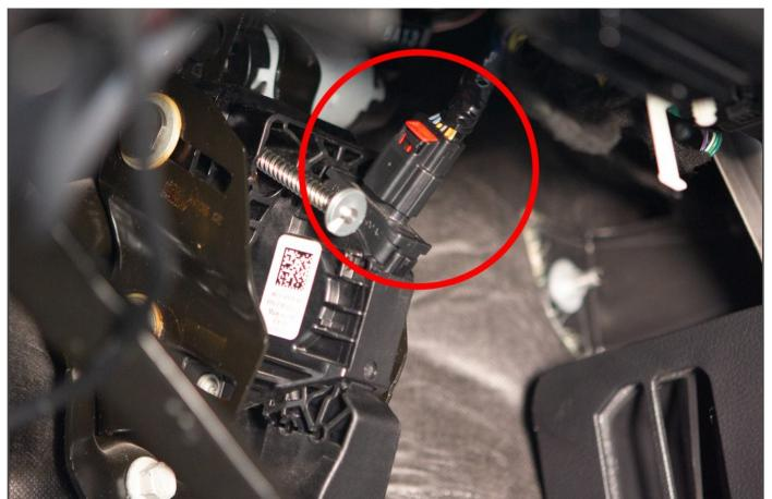
3. If the connector has a locking tab, slide the locking tab outwards to unlock. This will expose a black plastic button you will pinch to unlatch. Remove the connector from the accelerator pedal.
